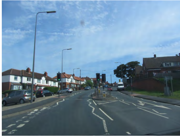
Photograph 25. A171 Helredale Road looking south leaving Whitby. Load moves away from camera. 5m clearance between lights and railings. Negotiable.
