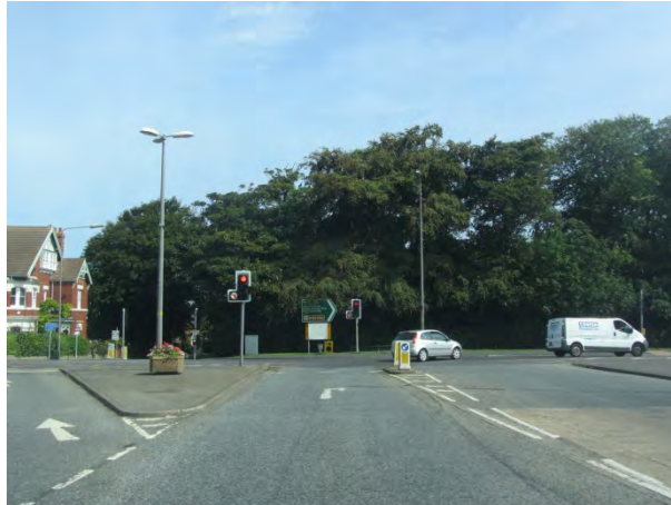
Photograph 20. A171/A174 Prospect Hill junction in Whitby. Contraflow recommended on the northbound slip road to avoid removal of street furniture if the load was to travel in a conventional fashion.
